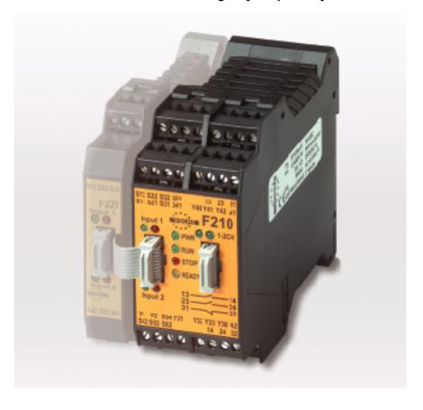
either an appropriate E-stop or fault condition occurs. The status of inputs/ outputs and diagnostic information are indicated by LED lamps, signalled by relay contacts and semiconductor outputs, and also transmitted through a serial data interface on the front of the Module.
